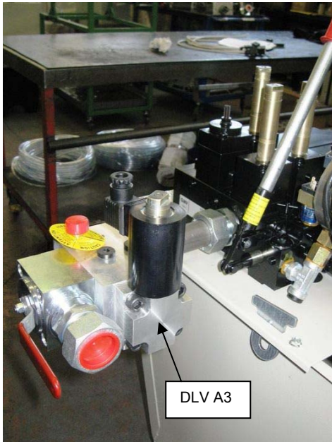
Typical DLV A3 assembly with shut off valve ≤ 150 litres
